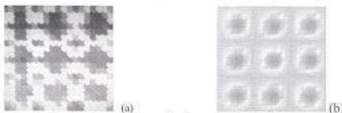
Fig.1. (a) Tomographic reconstruction of membrane transverse vibration amplitude; (b) 2D-map of membrane transverse oscillation (3,3)-eigenmode (theoretical calculation).
